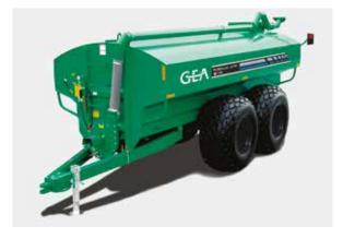
The GEA tandem is designed with a full length central tube, providing more resistance to twisting than conventional open tandem axles. The "V" shape design lowers the reservoir, lowering the center of gravity and increases stability. With this design, the wheels are located closer to the reservoir, reducing the flex on the axle.
